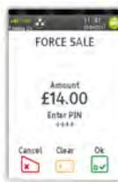
The terminal will request the PIN code. Cardholder to enter the PIN and then press
