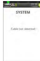
This screen will be displayed if the terminal cannot detect the network cable on the base.
