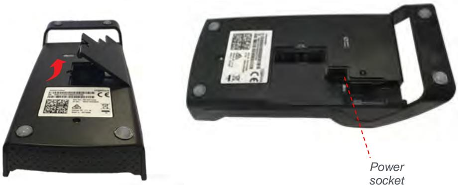
**Bluetooth Base: Is used for charging the terminal battery and has ports to allow terminals to communicate with hosts over Ethernet.**
