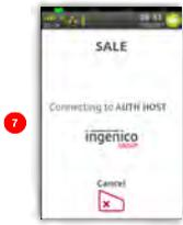
7 Terminal connects to the acquirer using the configured connection method e.g. 'Mobile Network'.
