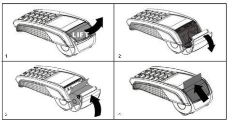
1. Hold the terminal securely in one hand. With the other hand, and by using two fingers, lift the printer cover release as shown. Fully open the printer cover and remove the old roll of paper.
