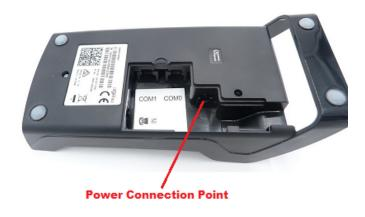
Once the Base is connected, place the terminal in the charging base and allow the device to power up. This will take approximately 2 minutes.
