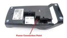
Once the Base is connected, place the terminal in the charging base and allow the device to power up. This will take approximately 2 minutes.
