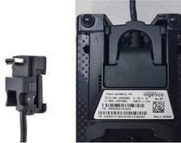
Connect the Power supply to the Terminal cable, and connect to an active Ethernet port. \*Note the Ethernet extension block and additional cable can be used to extend the cable if required.
