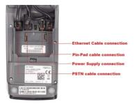
Once the Base and any additional cabling is connected, allow the device to power up. This will take approximately 4 minutes.
