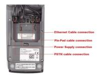
Once the Base and any additional cabling is connected, allow the device to power up. This will take approximately 4 minutes.
